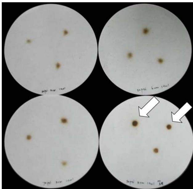
**Fig. 2** Ten microliters of brown pigment as loading buffer generates the best impact area with 50 psi, with the target at 3 cm (*bottom right; arrow*). Other conditions tested were 30 psi, 3 cm (*upper left*); 70 psi, 3 cm (*bottom left*), and 50 psi, 6 cm (*upper right*)
