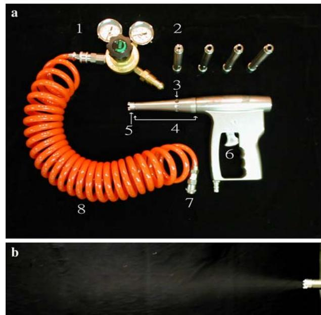
**Fig. 1** BioWare low-pressure gene gun and image of sample explosion from the gun. **a** Low-pressure gene gun and its accessory parts, 1 regulator; 2 barrels with different inside diameter; 3 loading aperture; 4 sleeve; 5 spacer; 6 trigger; 7 quick coupling; 8 PU coil tube. **b** Pattern of bursting mist from the gun at 50 psi helium pressure in 20  $\mu$ l distilled water simulation
